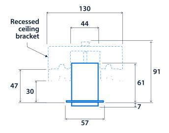
Mounting Arrangement -Plasterboard ceiling
