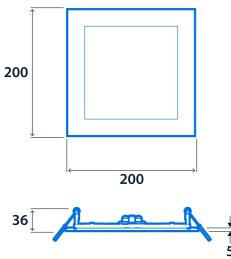
Cut-out - 180 x 180mm Minimum void depth: Standard - 40mm Smart & Emergency - 90mm
