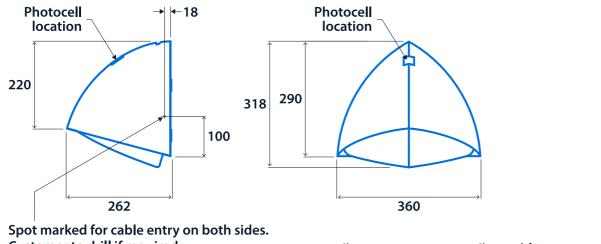
Spot marked for cable entry on both sides. Customer to drill if required.
