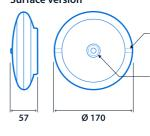
**Surface version** Side conduit entries (drill as required) Ø 21 cable entry
