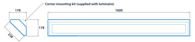
NOTE: Supply entries and fixing points to be drilled on site. IP66 integrity must be maintained
